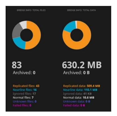
Two pie charts display the distribution of data within the workspace volume(s) depending on its Bridge status respectively by number of files and by data size.
